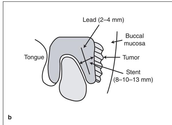
**Figs 2a and 2b** (a) Mandibular assembly with acrylic resin stent and lead shield cover. (b) Schematic representation of the stent with lead shield.
