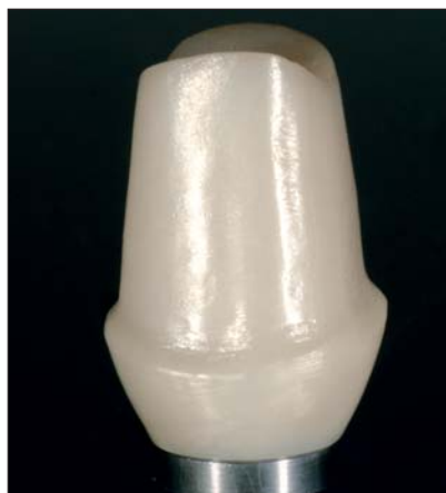
Fig 1 (left) Zirconia closure margin on the metallic abutment (group 1).
