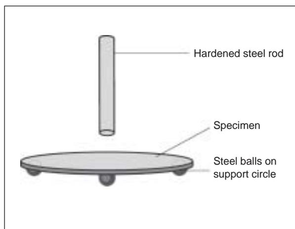
**Fig 1** Piston-on-3-ball setup for the biaxial flexural strength test.
