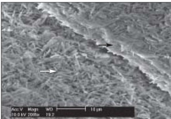
**Fig 7** SEM image of etched Empress 2 specimen ( $\times 2,085$ ) (white arrow: pinnacle-shaped lithium disilicate crystals; black arrow: lithium disilicate crystals embedded in glass matrix).
