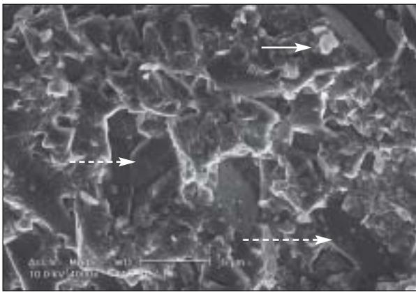
**Fig 3** SEM image of unetched In-Ceram Zirconia ( $\times 4,000$ ) (solid arrow: zirconia polycrystal; dashed arrows: alumina platelet).
