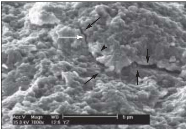
**Fig 5** SEM image of unetched YZ Zirconia ( $\times 7,000$ ) (black arrows define the pathway of a crack; white arrow: intergranular fracture; arrowhead: transgranular fracture).
