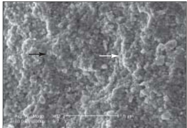
**Fig 6** SEM image of unetched Cercon ( $\times 7,000$ ) (white arrow: aggregates of tetragonal zirconia granules; black arrow: conglomerates appearing to be monoclinic zirconia).
