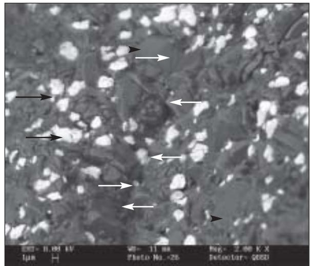
**Fig 4** SEM image of etched In-Ceram Zirconia (backscattered image,  $\times 2,000$ ) (black arrows: zirconia polycrystal; arrowheads: alumina plate; white arrows define the pathway of a crack).
