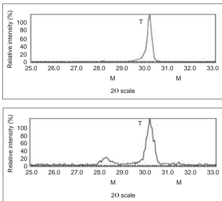
fractured YZ Zirconia surface contained approximately 5 times as much monoclinic phase compared to that of its intact surface. The fractured IZ and Cercon surfaces contained approximately twice as much monoclinic phase compared to their intact surfaces (Table 3).
