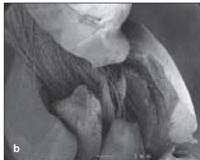
Figs 2a to 2d Representative specimen photographs ( a and c ) and SEM images after the fracture strength test ( b and d ). Note the delamination of the veneering resin into 2 primary pieces in FRC1 ( c ) and the catastrophic delamination of the veneering resin in FRC4 ( d ). (Original magnification \times 10 .)
