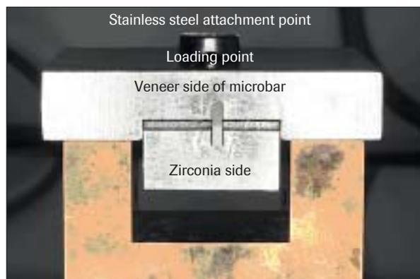
**Fig 2** Zirconia veneer microbar attached to the attachment unit using a light-polymerized adhesive resin. As the 2 plates of the attachment unit are separated, the interface is subjected to tensile stresses.
