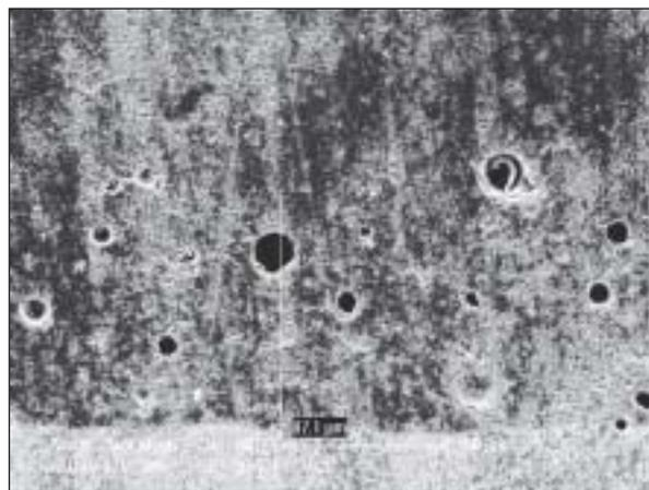
**Fig 5** SEM image demonstrating the structural defects and air bubbles at the zirconia-layered veneer interface. (Magnification  $\times 500$ .)
