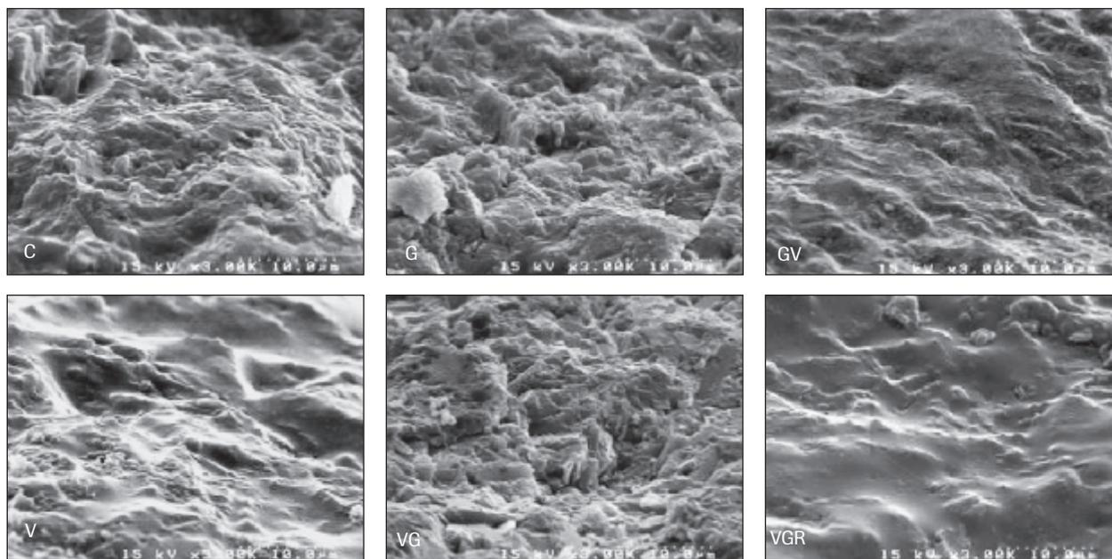
**Fig 1** SEM micrographs ( $\times 3,000$ ) of lithium disilicate core ceramics subjected to different surface treatments. C = control group (as pressed and delivered); G = ground with a diamond bur; GV = ground with a diamond bur, followed by simulated veneer firing; V = simulated veneer firing; VG = ground with a diamond bur after simulated veneer firing; VGR = ground with a diamond bur after simulated veneer firing, followed by re-glazing.
