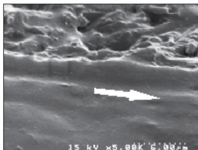
**Fig 2a (left)** Scanning electron micrograph ( $\times 5,000$ ) showing the surface flaws on a ground specimen (from group GV). White arrow = direction of grinding; gray arrow = multiple microcracks propagating perpendicular to the grinding direction.
