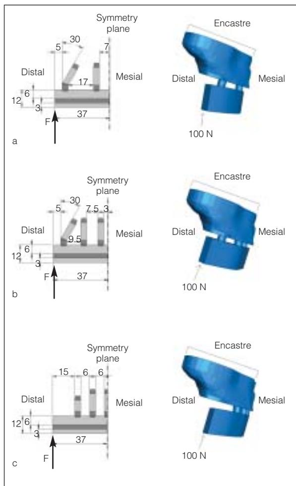
**Fig 1** Schematic drawings (*left*) and 3-D models including loading and boundary conditions (*right*) of the analyzed configurations: **(a)** All-on-4, **(b)** All-on-6, and **(c)** Toronto-Brånemark. Arrows indicate the point of application of the load (all measurements were recorded in mm).
