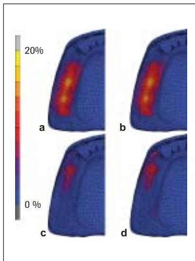
**Fig 3 (left)** Color coded stress distribution in the PDL for the indirect method with (a) Mini-SG PLUS and (b) MSG STAR, and for the direct method with (c) Mini-SG PLUS and (d) MSG STAR. The bar on the left indicates the color scheme used. Blue indicates zero stress while yellow indicates stresses of 10 MPa.
