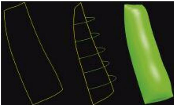
**Fig 5** Creation of the polished surface of a minor connector. **(left)** Outline of a minor connector. **(center)** Default cross section. **(right)** Polished surface generated using the component outline and the default cross section as restrictions.
