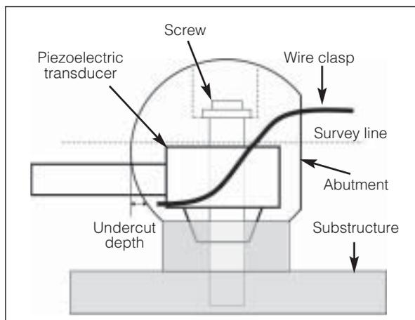
**Fig 2 (below)** Coordinates used for the analysis. The x- and y-axes run parallel to and the z-axis perpendicular to the pressure receiver of the transducer. A tested clasp was aligned along the y-axis and was removed upward along the z-axis. The positive direction of the x-axis is the side of the abutment with the clasp and the positive direction of y-axis is the side with the clasp tip. The positive direction of the z-axis is the upwards direction.
