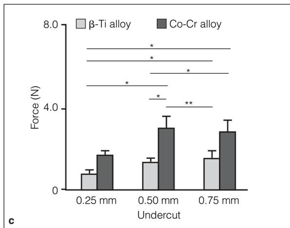
**Fig 4a** The maximum magnitude of the retentive force exerted on the abutment (z-axis). \* $P < .01$ .
