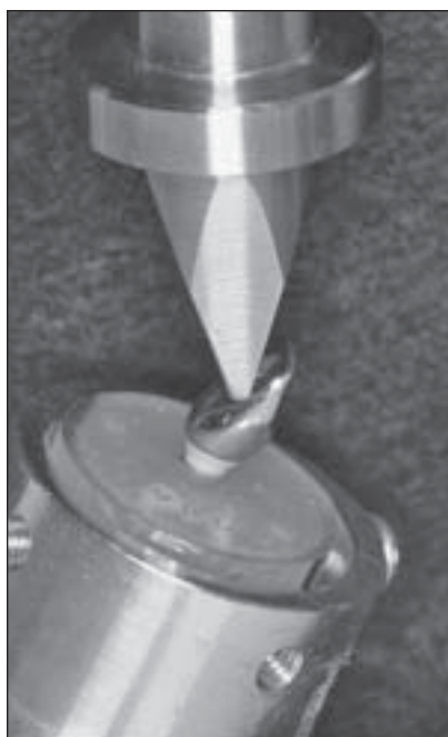
Fig 1 Specimen positioning and orientation at a 30-degree angle to the loading axis during accelerated fatigue testing.
