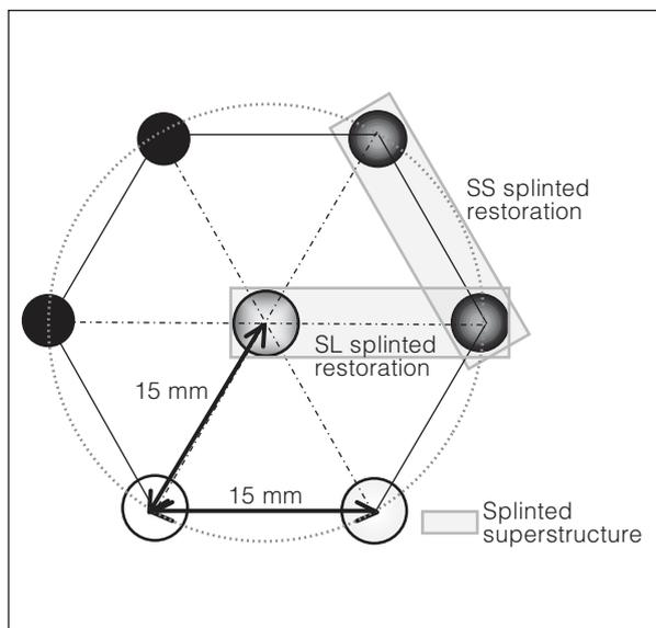
**Fig 1** Illustration of the test model configuration: 7-mm-long implants (short) of diameters 3.8 mm (black), 4.4 mm (gray), or 5.0 mm (white) were arranged at the apices of a regular hexagon. In the center of the hexagon was a 4.4 × 12.0-mm implant. Because it was a regular hexagon, the length of each superstructure in the SS and SL splinted restorations were the same.
