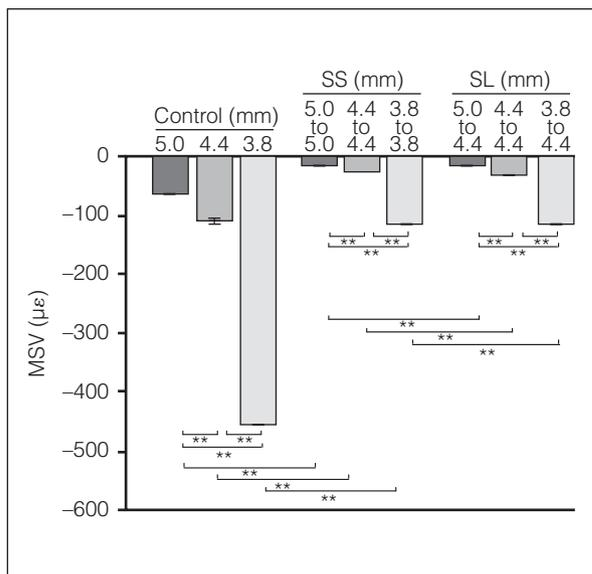
Mean strain values (MSVs) obtained from an average of the output from the strain gauges were compared using analysis of variance and post hoc analysis (*P* < .05; SPSS 11.0, IBM).
