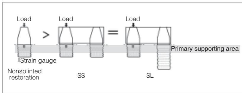
**Fig 4** Strain in the nonsplinted restoration was significantly larger than that in the splinted restorations under the same load. The strain was identical in SS and SL splinted restorations. The primary supporting area was identified below the platform and around the neck of the implant, which influenced the strain around the implant under loading.
