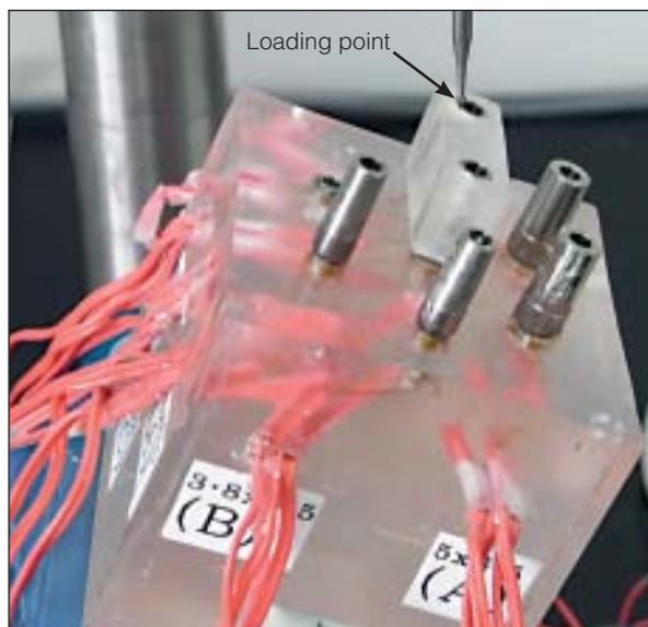
**Fig 2** Loading point and test on the splinted restoration (SL: 4.4 × 7.0 mm to 4.4 × 12.0 mm).
