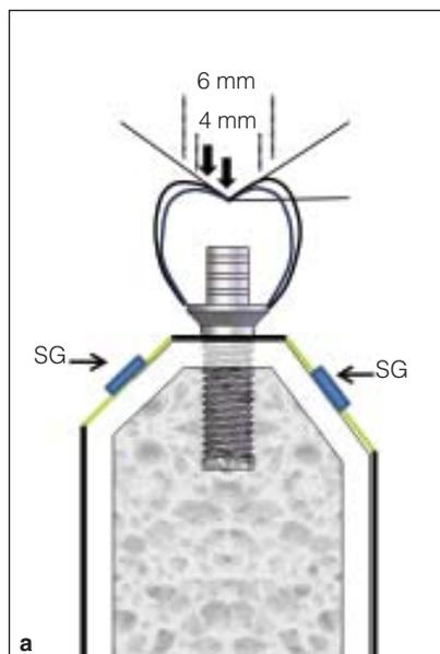
**Fig 1a** Experimental design for an implant-supported single crown with strain gauges (SG) attached at the buccal and lingual aspects.
