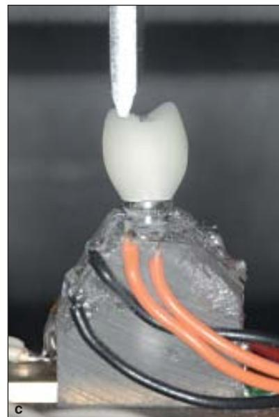
**Figs 1b and 1c** The applied forces were loaded at two sites: **(b)** the central fossa area and **(c)** 2 mm buccal to the central fossa.
