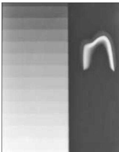
**Fig 1** Radiographic image of the aluminum stepwedge and a Cercon specimen slice.
