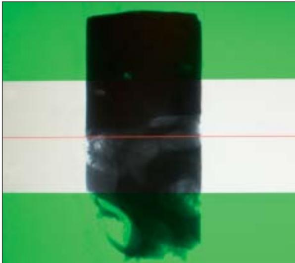
**Fig 2a** VOI measured from the middle of the specimen to 1 mm on both sides of the midline.
