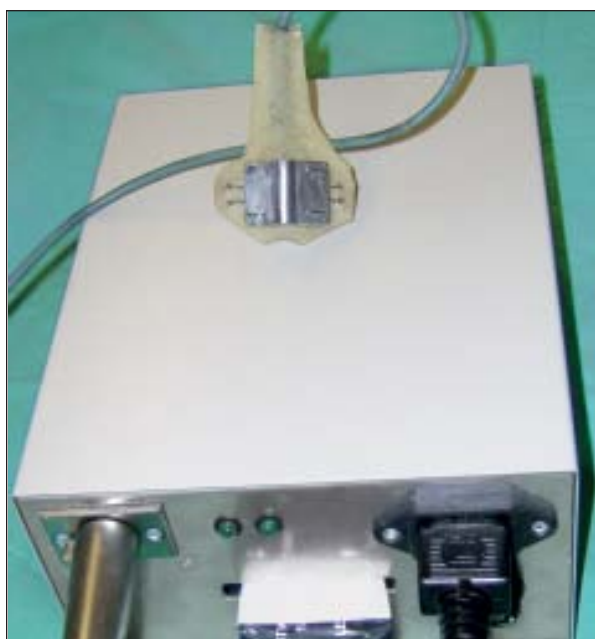
Fig 2 A data acquisition plaque was connected to a computer, and through use of software, mean retention values were able to be read.
