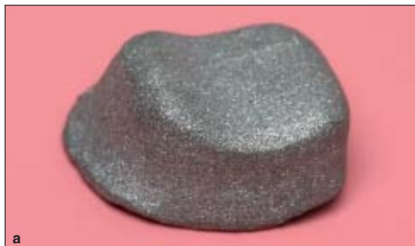
Fig 2 (a) Occlusal and (b) inner surfaces of a metal coping fabricated using laser-sintering technology.
