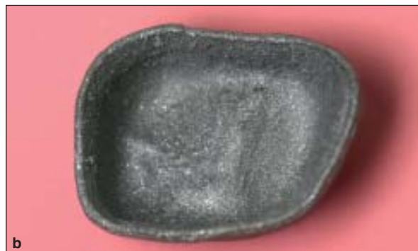
Fig 2 (a) Occlusal and (b) inner surfaces of a metal coping fabricated using laser-sintering technology.
