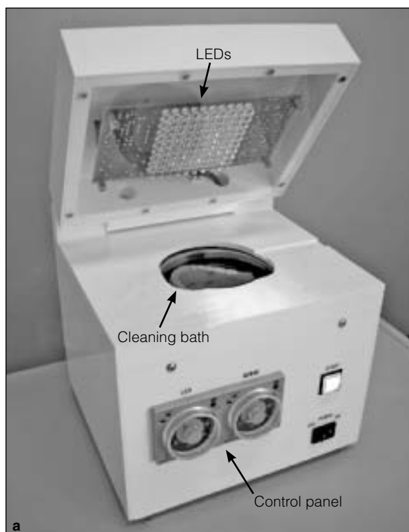
Figs 1a and 1b Experimental denture-cleaning device. A removable dental prosthesis is immersed in the cleaning bath containing 150 mL of 500 mM \text{H}_2\text{O}_2 and is then irradiated using the LED light and ultrasound.
