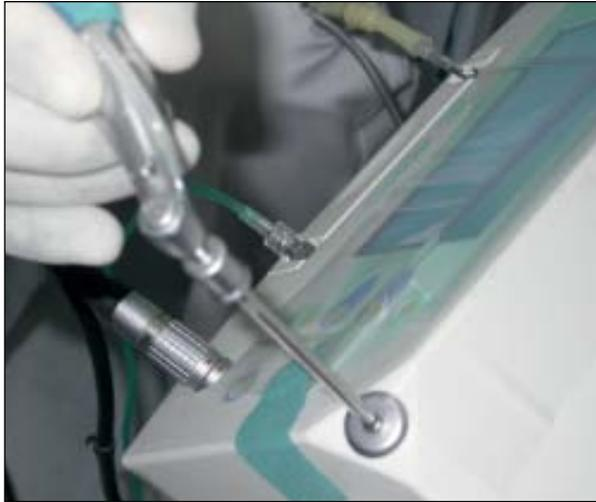
**Fig 1** Calibration of torque on the Elcomed motor.
