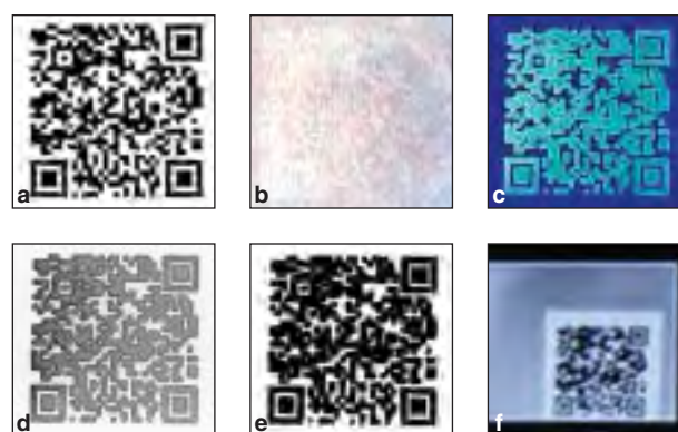
Fig 3 Two-dimensional QR code recording and reading. (a) Development of the QR code; (b) information recording on the resin surface; (c) QR code scanning; (d) image processing to gray image; (e) image processing to binary image; (f) QR code reading screen using a smart phone.
