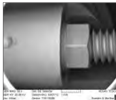
Fig 3 SEM image of abutment/screw complex after Argon plasma cleaning; note the absence of micropollutants (original magnification \times 50 ).
