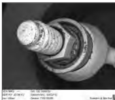
Fig 2 Scanning electron microscopy (SEM) images of abutment/screw complex after steam cleaning; ( left ) lateral and ( right ) apical views (original magnification \times 50 ).
