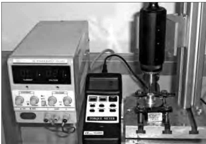
Fig 4 The measurement device with aluminum implant holder and the coaxial holder of the screw-driver joined to the torque meter and the electric engine.
