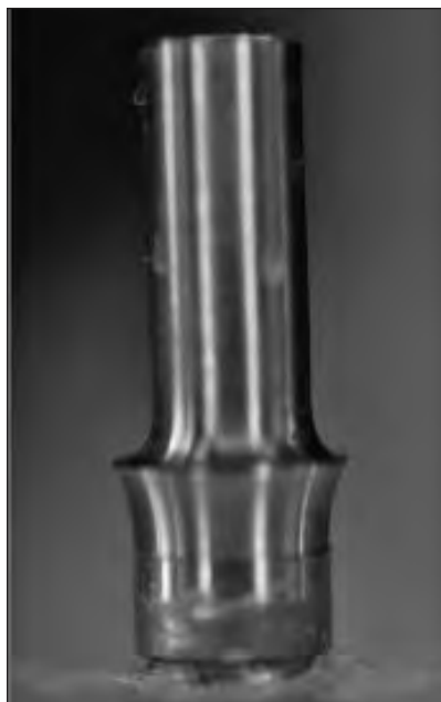
Fig 1 The titanium abutments ( left ) before and ( right ) after customization by means of carbide burs (coarse and fine) followed by steam cleaning.
