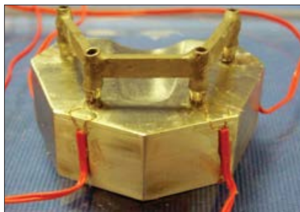
Fig 1 The metal framework seated on the master metal cast (1 to 2 and 3 to 4 = 28 mm, 2 to 3 = 26 mm).
