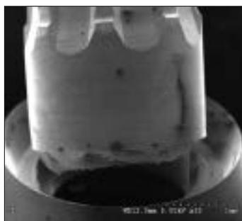
**Fig 4** SEM micrograph of an abutment fracture (magnification  $\times 35$ ).
