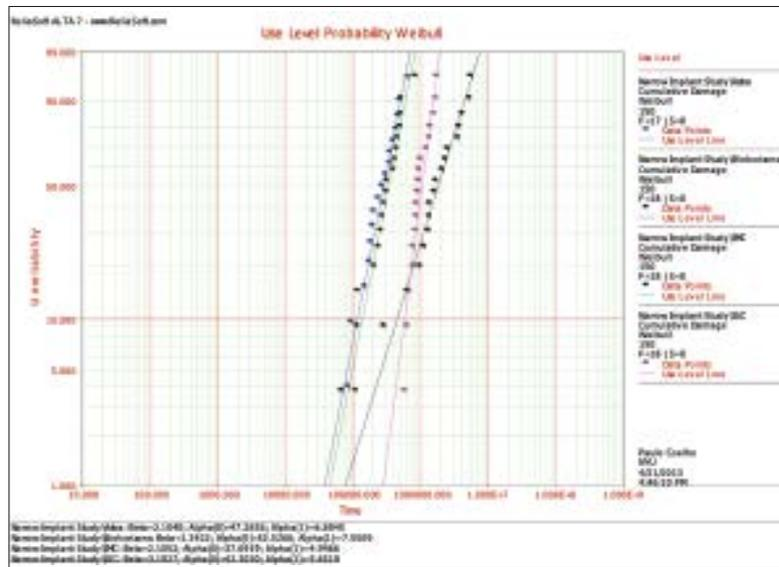
**Fig 2** (right) Use-level probability Weibull curve showing the probability of failure as a function of number of cycles (time) for 100,000 cycles at 150 N.
