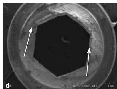
**Fig 5 (right)** SEM micrographs of representative fractures after SSALT. **(a)** Long-axis view of fractured abutment screw in group ASC; the arrows point toward the compression curl, while the opposite tensile side indicates its origin. The angulations of the arrows indicate the direction of crack propagation. Failure in groups **(b)** BSC, **(c)** ISC, and **(d)** IMC involved the same failure pattern.
