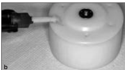
Fig 2 Specimen preparation. (a) Tablets were placed on the lower part of a polyamide mold. (b) After primer application, the upper piece of the mold was positioned and secured using a central screw, then a layer of luting cement was placed in the cavity (3.3 mm in diameter) and light cured. After polymerization, the cavity was filled with composite and light cured again.
