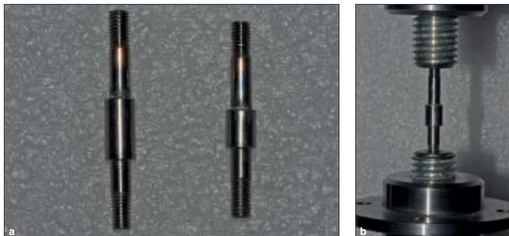
Fig 2 (a) Samples used during the investigation; (b) Instron machine during testing.
