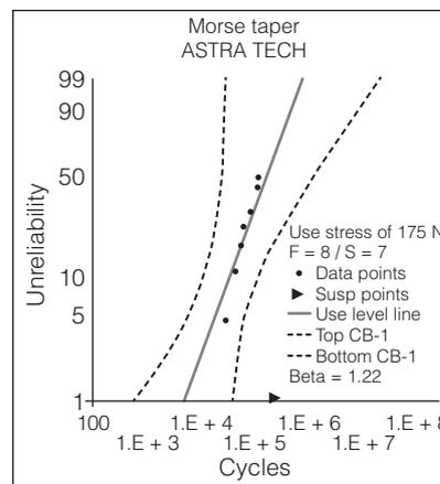
**Fig 2** Use level probability plots for both groups. Note that the Morse taper (MT) group showed Weibull  $\beta = 1.2$  and the cone fit (C) group presented  $\beta = 0.17$ .
