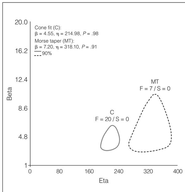
**Fig 3** Weibull probability calculation represented as contour plot showed Weibull modulus  $\beta = 4.55$  and characteristic strength  $\eta = 214.98$  for cone fit (C), and  $\beta = 7.20$  and  $\eta = 318.10$  for Morse taper (MT) abutments.
