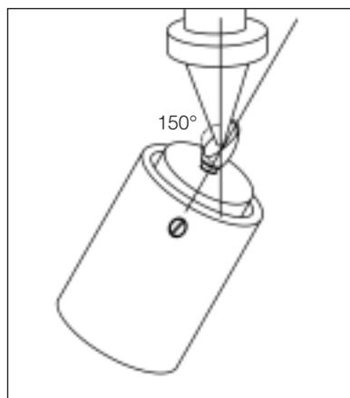
**Fig 1** This schematic representation shows the specimen positioning and orientation at a 30-degree angle to the loading axis. Note that the indenter is located at the midlingual aspect of the central incisor alloy crown.
