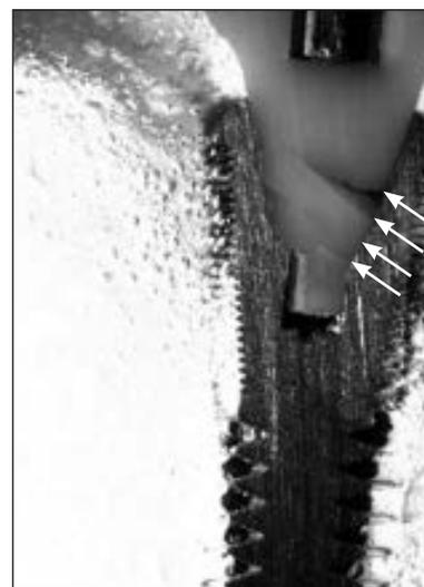
**Fig 5** Sectioned image of a failed Morse taper (MT) specimen with a fracture at the MT part of the abutment. White arrows point to several cracks formed as a result of the fatigue employed.
