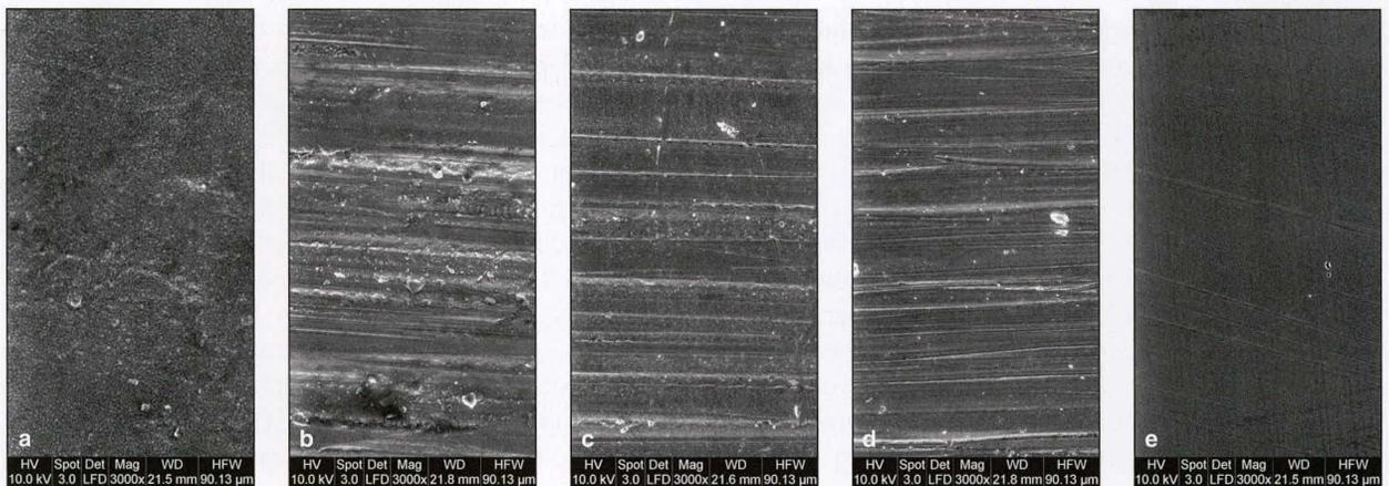
**Fig 1** Scanning electron microscopy images (magnification:  $\times 3,000$ ) of zirconia after (a) sintering, (b) grinding, (c) polishing step 1, (d) step 2, and (e) step 3. Example from three-step intraoral polishing kit (CeraGlaze).
