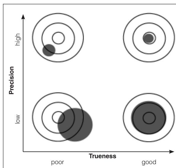
Fig 4 The difference between precision and trueness. The top-right diagram depicts high accuracy.
