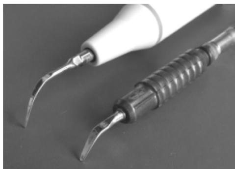
Fig. 1. The scaler tips used in this investigation including (left) a P-style piezoelectric tip and (right) a TFI-3 magnetostrictive tip.
