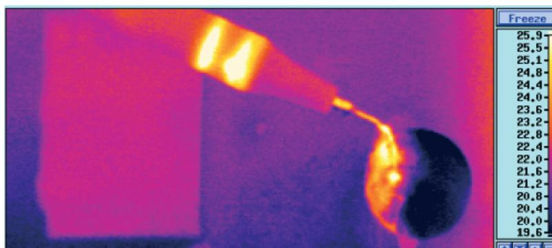
Fig. 3. A typical thermal image obtained using the Agema 900 Thermal Imaging System, for the Mini Piezon, after approximately 40 s of instrumentation. A hotspot is observed at the tip/tooth contact site and an increase in temperature is also seen for the scaler handpiece where the piezoelectric crystal is located.
