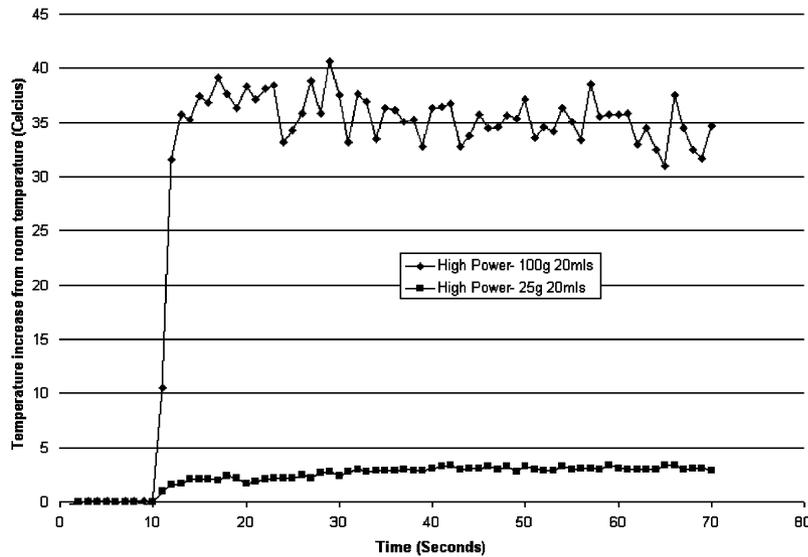
Fig. 4. Graphs of increase in temperature with time for the Mini Piezon scaling system, demonstrating the effect of contact load on temperature. The mean background temperature was calculated and subtracted from all data, enabling the increase in temperature, from room temperature, to be observed. Instrumentation conditions are high generator power setting and 20 ml/min water flow rate with loads of 25 g, 50 g and 100 g.
