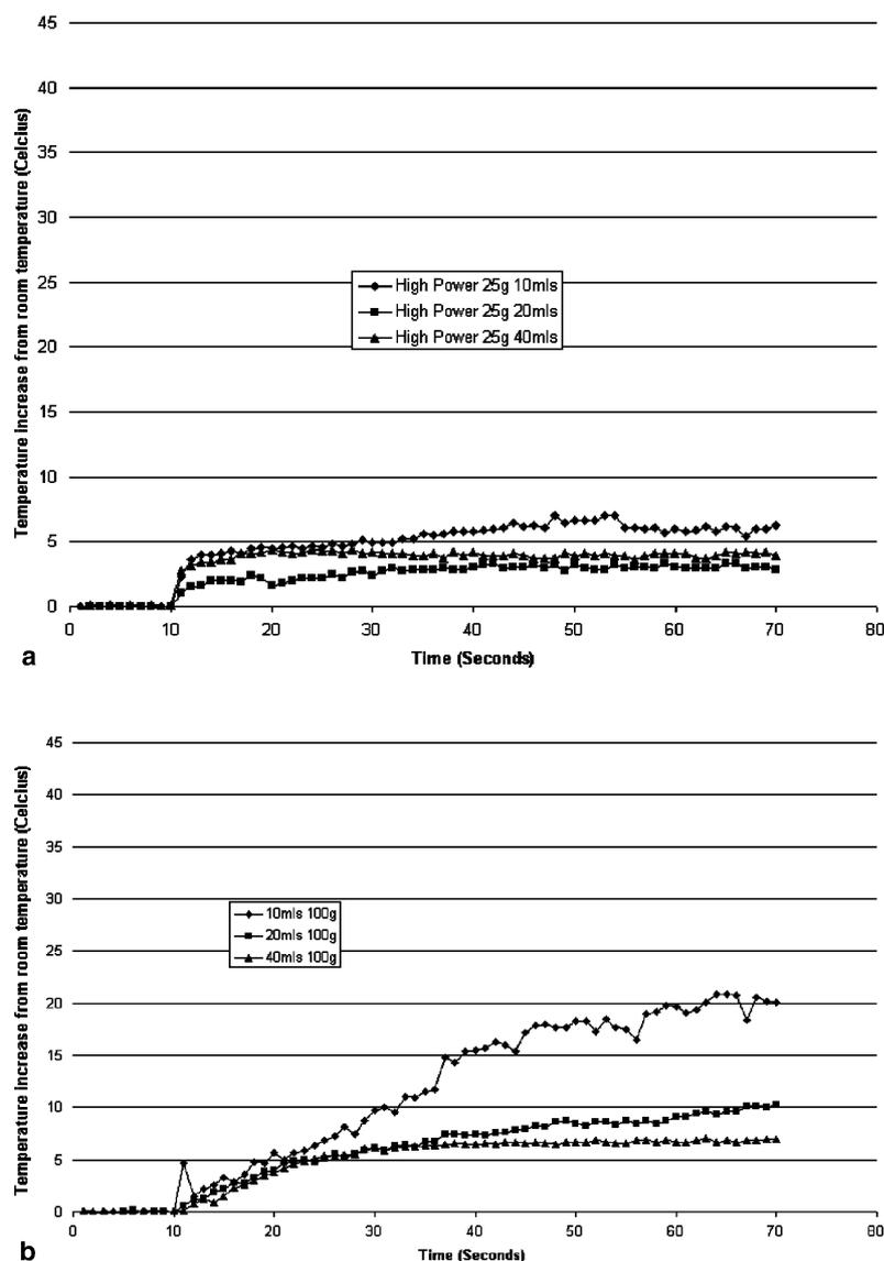
Fig. 6. Graphs of increase in temperature with time, demonstrating the effect of water flow rate on temperature. Instrumentation conditions are (a) Mini Piezon; high power/25 g load/10, 20 and 40 ml/min water, (b) SPS; medium power/100 g load/10, 20 and 40 ml/min water and (c) Mini Piezon; high power/100 g load/20 and 40 ml/min water.
