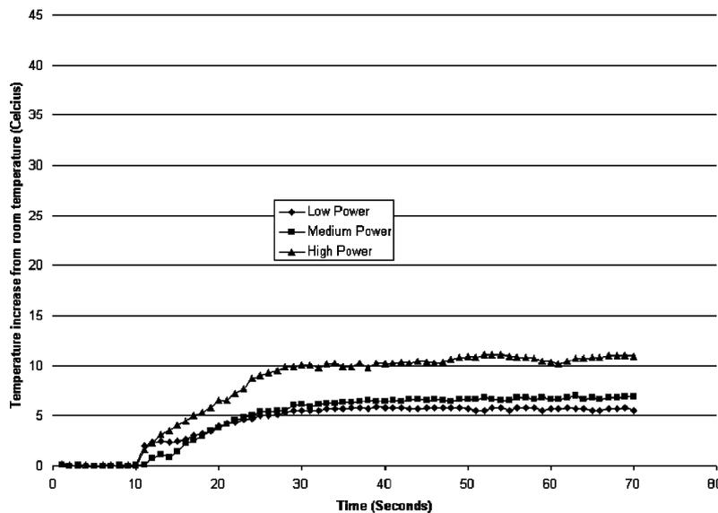
Fig. 5. Graphs of increase in temperature with time for the SPS scaling system, demonstrating the effect of generator power setting on temperature. Instrumentation conditions are 100 g load and 40 ml/min water flow rate with generator power settings of low, medium and high.
