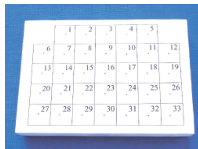
Fig. 3. This construction was then covered with plaster of Paris, leaving only the probing faces uncovered.
