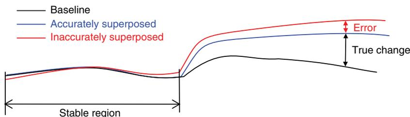
Fig. 8. Inaccurate superposition and its effect on measured changes.
