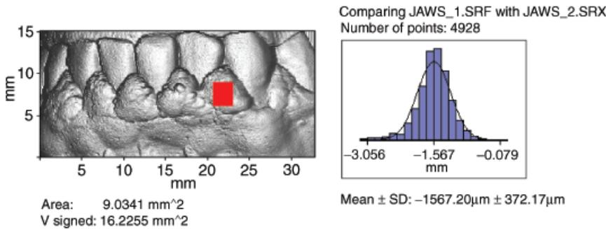
Fig. 7. Measurement of change over a selected rectangular region of 9 mm<sup>2</sup>, showing a total volume loss of 16.2 mm<sup>3</sup> over that region. The mean depth loss over that region was 1.567 mm.
