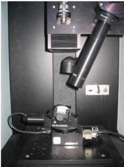
Fig. 1. Laserscan 3D Pro system with model in situ.
