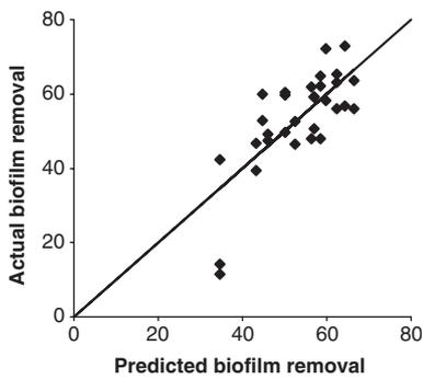
Fig. 3. Plot comparing actual biofilm removal data (individual points) to the predicted biofilm removal values from the mathematical model. The solid line is a guide to the eyes showing a  $y = x$  line.
