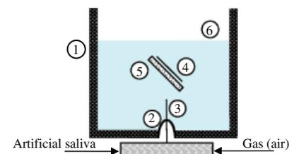
Fig. 1. Schematic of the experimental chamber. (1) Plexiglas chamber, (2) rubber septum, (3) 25-gauge needle, (4) biofilm on glass coverslip, (5) glass slide acting as a shutter, and (6) artificial saliva level.
