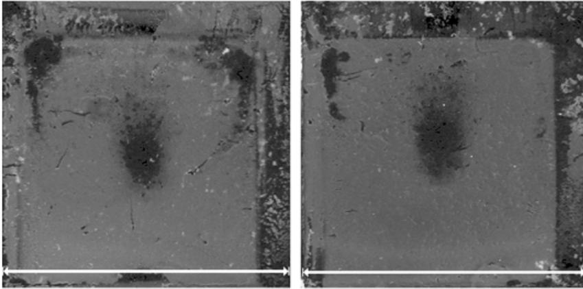
Fig. 4. Biofilms after exposure to bubble streams of different gas fractions. Left, velocity of the stream was 10.1 m/s, gas fraction was 0.55, and the bubble diameter was 257  $\mu\text{m}$ . Right, velocity of the stream was 12.2 m/s, gas fraction was 0.34, and the bubble diameter was 261  $\mu\text{m}$ . The white area is the biofilm and the black area in the centre is where the biofilm was removed. The scale bar represents 2.54 cm.
