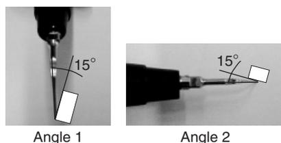
Fig. 3. Schematic drawing of the two angles tested for potential influence on surface recognition results. Angle 1 depicts the instrument's deviation from the longitudinal axis of the tooth (varied between 15° and 45°), whereas angle 2 stands for the rotation of the instrument along the distal tip axis (varied between 15° and 90°).
