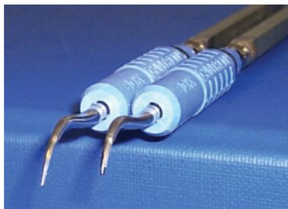
Fig. 2. An unaltered tip is placed alongside a tip that has been ground by 2 mm to simulate the effect of wear.
