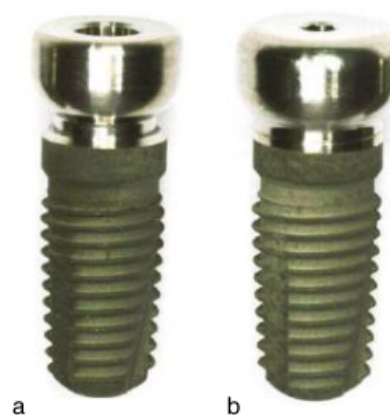
Fig. 1. (a) Platform-switching was created by connecting wide-diameter ( \varnothing 5.0 mm) test implants with smaller-diameter healing abutments ( \varnothing 4.0 mm), resulting in a circumferential horizontal mismatch of 0.5 mm. In particular, the circumferential plateau revealed an outer bevelled ( 45^\circ ) part of 0.3 mm, and an inner horizontal part of 0.2 mm. (b) Commercially available wide-diameter implants ( \varnothing 5.0 mm) with matching wide-body healing abutments served as control. Both types of implants had an identical design, exhibiting a machined-neck size of 0.4 mm.
