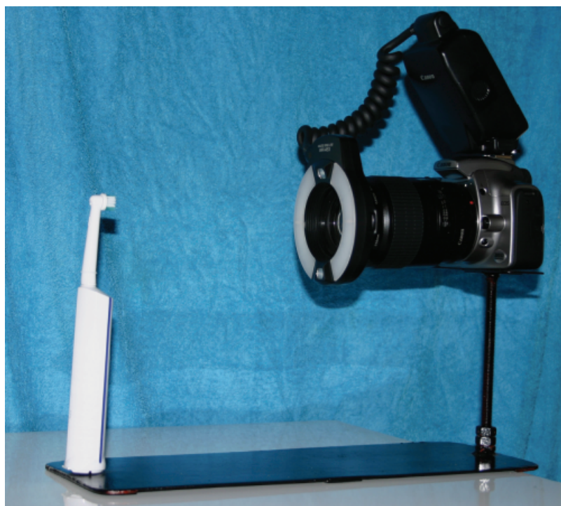
Fig. 1. Customized jig for taking standardized digital photographs of the brush heads.
