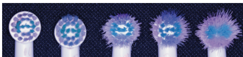
Fig. 2. Three-month-old brush heads exhibiting variations in bristle wear. The percentage increase in brushing surface area for the illustrated brush heads was (from left to right) 0%, 16%, 46%, 72% and 94%.
