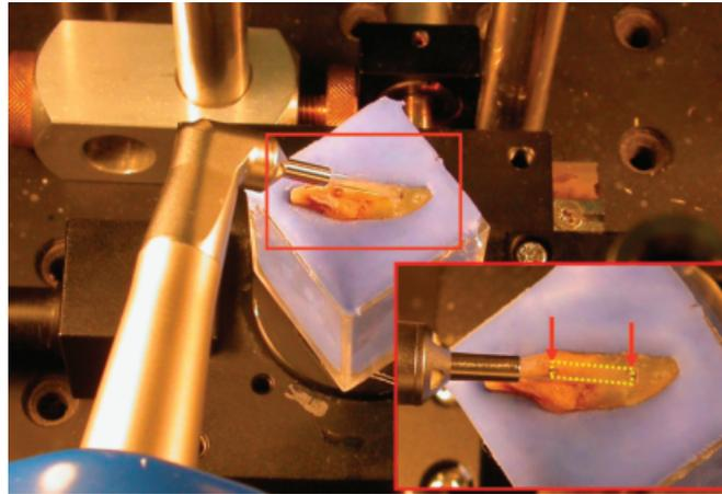
Fig. 1. Experimental set-up. Teeth and handpiece of the Er:YAG laser fixed on a translation stage. The angulation between the chisel-shaped application tip and the root surface was 15°. Detail: the area of interest of the treated root surface was determined both by the diameter of the used application tip (yellow marking) and by small notches prepared in the coronal and apical part of the root surface (red arrows).
