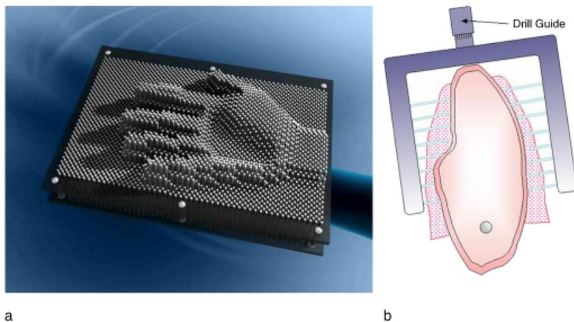
Fig. 2. (a) This simple “nail board” illustrates the idea of the micro-needle array for registration of the bone surface. By means of the matrix of needles a three-dimensional image of a surface can be generated. (b) The technical realization of the “nail board principle” on the jaw bone is accomplished by means of the bone surface imaging needle array.
