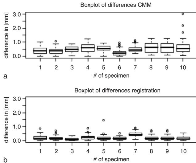
Fig. 8. Boxplots of all results at the 10 specimen for (a) the coordinate measuring machine measurements and (b) the bone surface imaging needle array registration. Boxplots showing first and third quartile (i.e. the box is the interquartile range) and median, the lines (‘‘whiskers’’) depict the 1.5 × interquartile range above and below the hinges of the box, circles indicate outliers.
