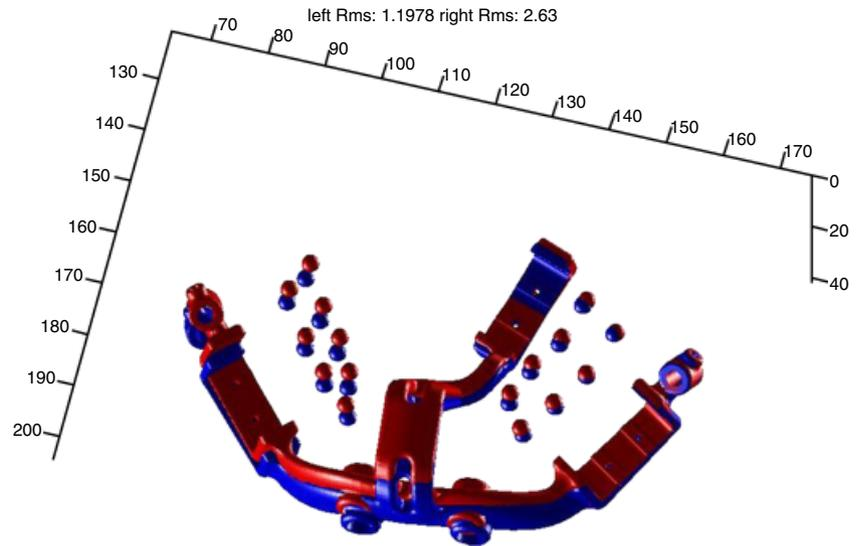
Fig. 7. The frame with the probe points at both sides. Depending on the ‘‘area of interest’’ for the evaluation of the registration (i.e. the location of the planned implant insertion) our data for the analysis are based on left or the right set of points. In this example the frame is oriented onto the left side, therefore in this example registration is better on the left side and only these eight points from the left side are considered in the performance analysis.
