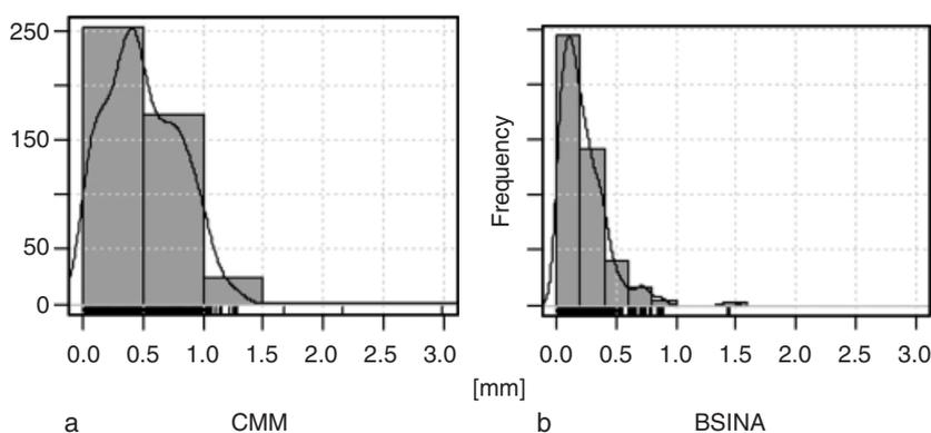
Fig. 10. Histograms illustrate the frequency of the observed errors. With the bone surface imaging needle array (a) smaller errors were measured more frequently as compared with the coordinate measuring machine (b).
