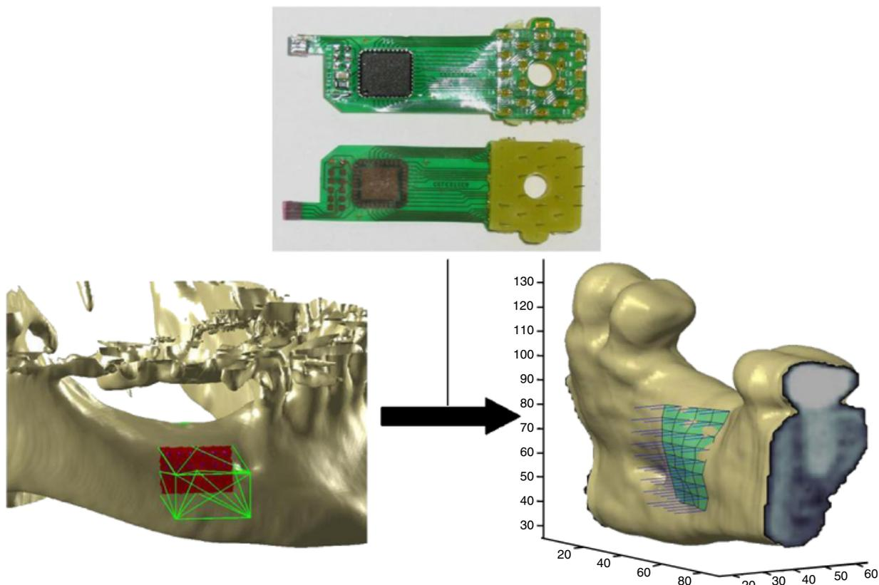
Fig. 5. The needles of the bone surface imaging needle arrays (attached to the jaw using the frame) are driven by push–pull hydraulics to penetrate the soft tissue, stopping when their tips touch the surface of the bone. The electronic device generates the points for the surface matching.
