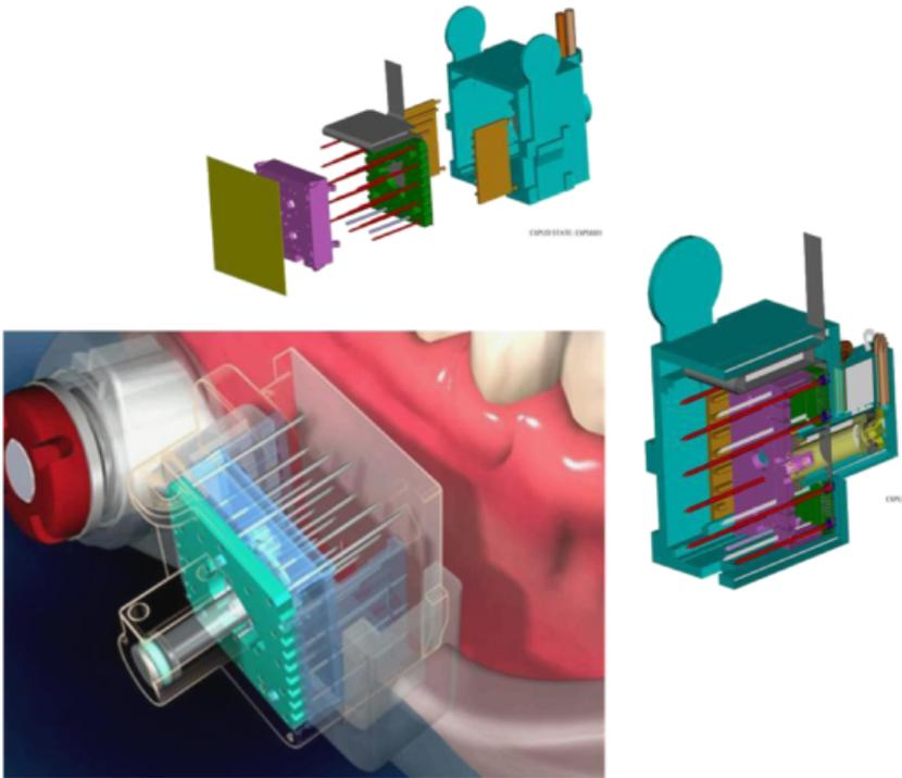
Fig. 3. Exploded drawing of the array of micro-needles, which is embedded in a cartridge.
