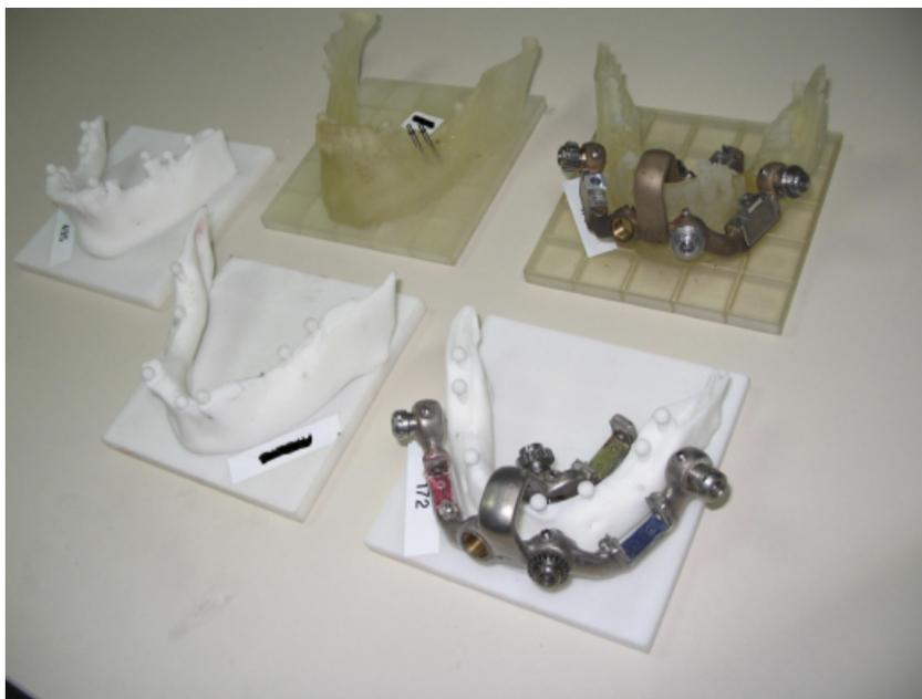
Fig. 6. Figure shows some of the jaw models (two of them already supplied with prototypes of the frame) as used for the registration experiments.
