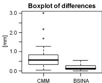
Fig. 9. Boxplots summarize the measurements at the 10 specimen with the bone surface imaging needle array (right Boxplot) and the coordinate measuring machine (left Boxplot).
