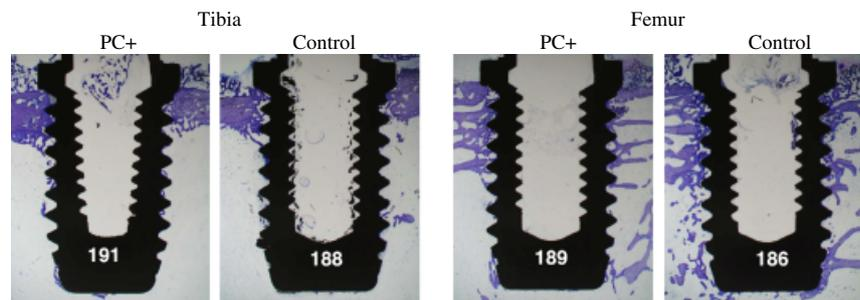
Fig. 3. Representative photomicrographs of implants coated with positively charged phosphorylcholine (PC+) and control.
