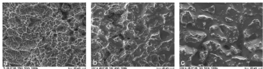
Fig. 2. SEM pictures of the implant surfaces: (a) sandblasted acid-etched titanium, (b) collagen/chondroitin sulphate (CS1), (c) collagen/CS2. Images were acquired with 1 kV for protein-coated samples with no additional surface preparation (LEO Gemini DSM 982).
