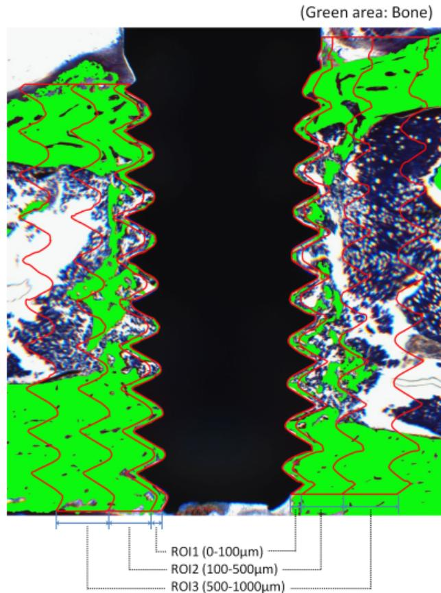
Fig. 2. Bone fraction analysis. The amount of bone in three different regions of interest (ROI) is measured. These regions differ in their distance to the implant. ROI1: 0–100  $\mu\text{m}$ , ROI2: 100–500  $\mu\text{m}$  and ROI3: 500–1000  $\mu\text{m}$ .
