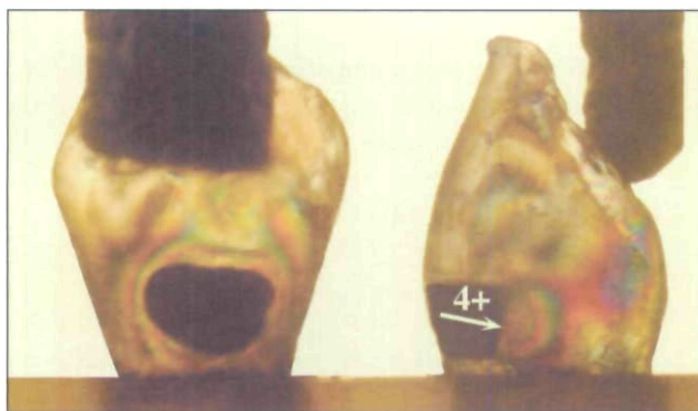
Figure 8. Low preparation with high modulus restorative under a cingulum load of 10 lbs.
