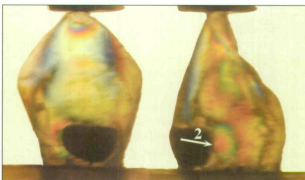
Figure 5. Low preparation with low modulus restorative under a cuspal load of 10 lbs.
