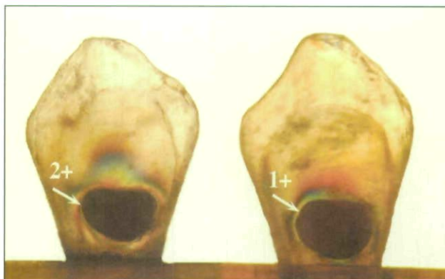
Figure 3. Polymerization shrinkage stresses. Left: high modulus restorative; right: low modulus restorative.
