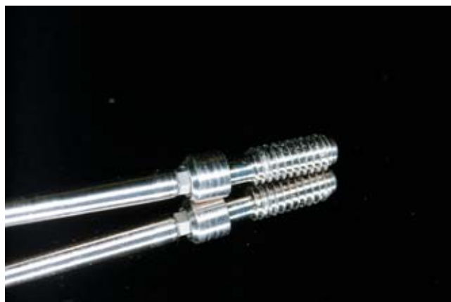
Figure 5. Following the milling, the screwdriver shank can be used to engage the abutment screw through a very small access hole in the crown.
