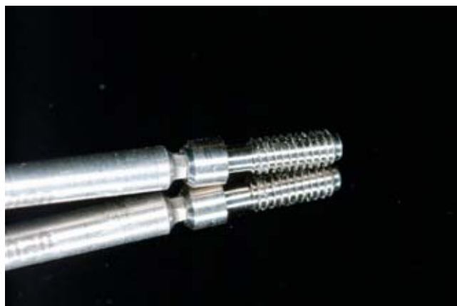
Figure 4. A screwdriver in its original diameter will require a large hole in the final crown, and accommodating it will result in an offset position of the implant.
