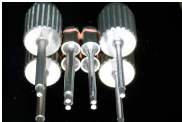
Figure 3. The shanks of the two screwdrivers on the left were milled to the diameter of the mating surfaces on the abutment screw (the two screwdrivers on the right).
