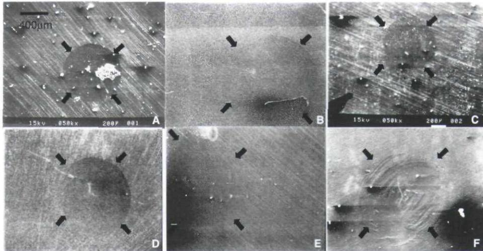
Figure 6. Scanning electron micrographs of enamel specimens worn against respective materials ( $\times 50$  original magnification): A, SureFil; B, Alert; C, Solitaire; D, Pyramid; E, TPH; F, Dispersalloy. Arrows indicate borders of wear. Note that the surfaces against composites were quite smooth, whereas amalgam left some flaws.
