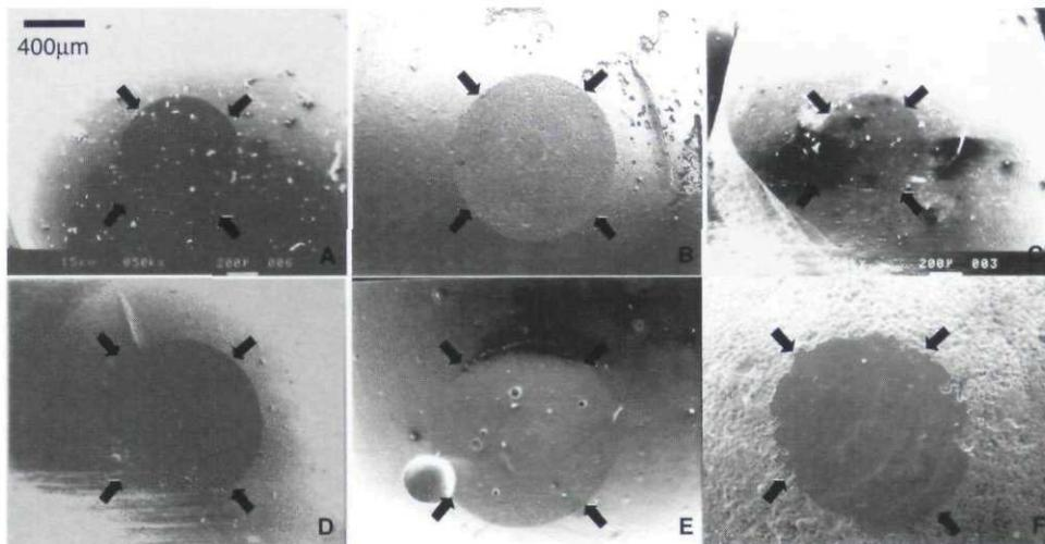
Figure 7. Scanning electron micrographs of material surfaces worn against the flat enamel surfaces ( $\times 50$  original magnification): A, SureFil; B, Alert; C, Solitaire; D, Pyramid; E, TPH; F, Dispersalloy. Arrows indicate borders of wear. Note that Alert specimen exhibited some filler exfoliation. Other composite specimens showed smooth surfaces, whereas amalgam left some flaws.
