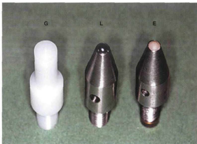
Figure 1. Styli for respective wear tests. G = generalized wear stylus made of polyacetal; L = localized wear stylus with stainless steel ball tip; E = enamel wear stylus with composite tip.
