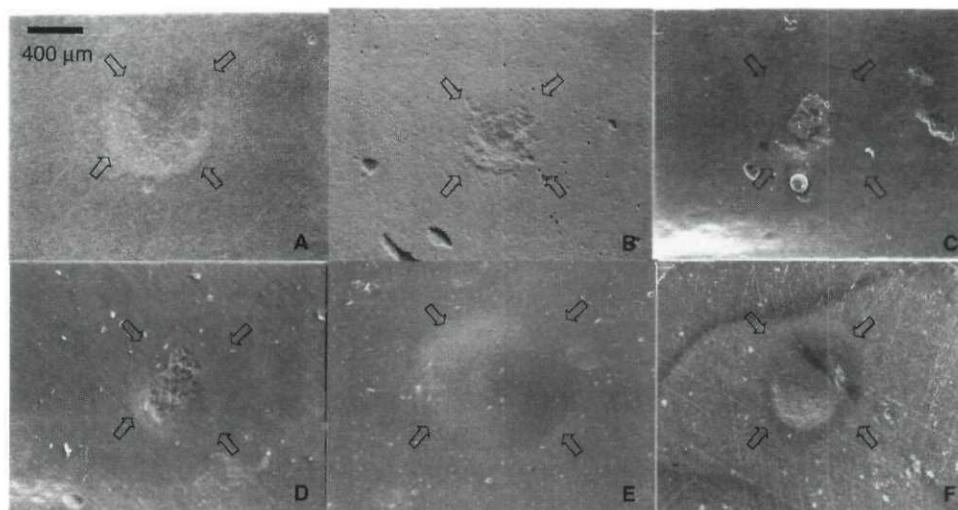
Figure 5. Scanning electron micrographs of the specimens after the localized wear test ( $\times 50$  original magnification): A, SureFil; B, Alert; C, Solitaire; D, Pyramid; E, TPH; F, Dispersalloy. Arrows indicate borders of wear. Note that cylindrical filler particles can be seen on Alert specimens. Clusters of wear debris remained on Solitaire and Pyramid after the wear process.
