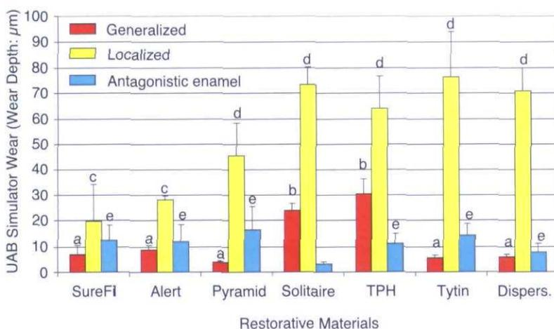
Figure 3. Results of the *in vitro* wear tests in a UAB wear simulator. Respective wear tests were completed with different types of styli. Error bars represent SDs. Bars with the same letters are not significantly different within the same wear mode ( $p \leq .05$ ).
