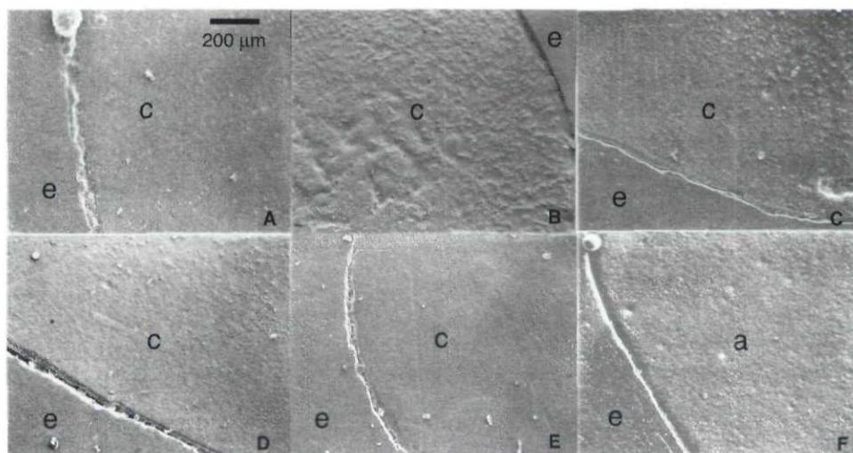
Figure 4. Scanning electron micrographs of worn surfaces after the generalized wear test ( $\times 100$  original magnification): A, SureFil; B, Alert; C, Solitaire; D, Pyramid; E, TPH; F, Dispersalloy. Note that individual filler particles can be seen on Alert, Solitaire, and Pyramid specimens. a = amalgam; c = composite; e = enamel.
