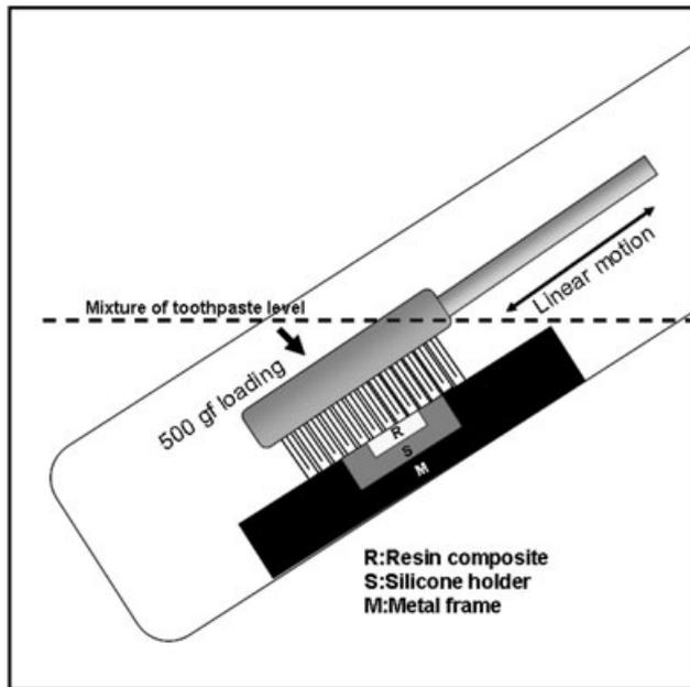
Figure 1. Diagram of brushing apparatus.
