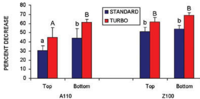
Figure 7. Percent decrease from maximum Knoop hardness of microfill (A110) and hybrid (Z100) composite resins on the top and bottom surfaces using the standard and turbo light guides.  $N = 5$  for each test condition. For a given composite and surface, use of the turbo tip provided a significantly greater decrease in hardness than did the use of the standard tip. Values denoted by similar lowercase (standard guide) or uppercase (turbo tip) letters are not significantly different.
