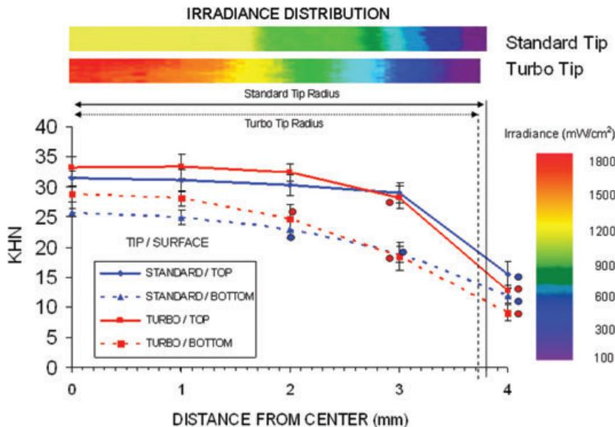
Figure 6. Hybrid composite resin (Z100) top and bottom surface hardness (Knoop hardness [KHN]) and corresponding power density distribution. KHN values at distances indicated by a colored circle are significantly different from that at the corresponding specimen center ( $p < 0.05$ ).  $N = 5$  specimens per group; vertical bar = 1 SD.
