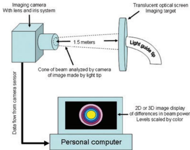
Figure 1. Diagram of the system for analyzing the curing light beam.
