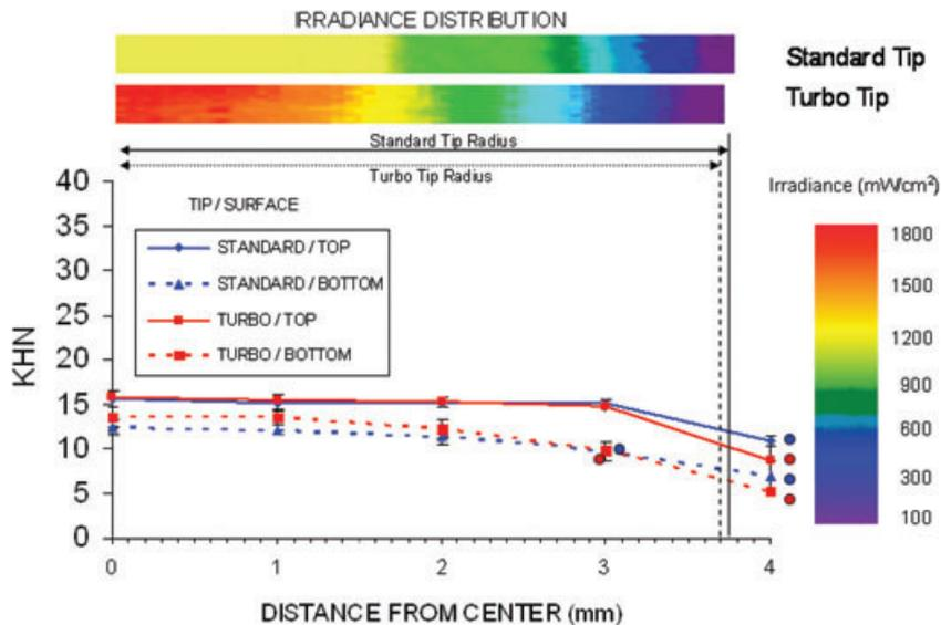
Figure 5. Microfill composite resin (A110) top and bottom surface hardness (Knoop hardness [KHN]) and corresponding power density distribution. KHN values at distances indicated by a colored circle are significantly different from that at the corresponding specimen center ( $p < 0.05$ ).  $N = 5$  specimens per group; vertical bar = 1 SD.
