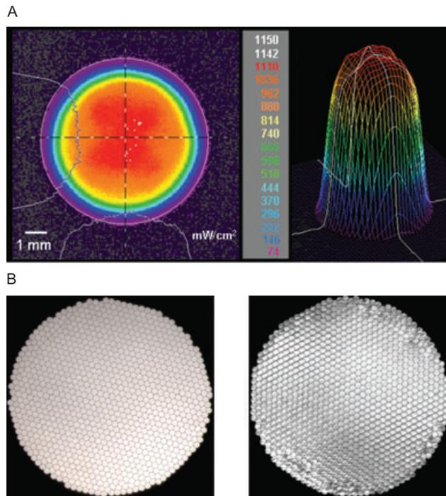
Figure 3. A, Two- and three-dimensional beam profiles across the standard light guide tip (0 mm) (Top Hat factor = 0.785) and corresponding irradiance values ( $\text{mW}/\text{cm}^2$ ). Total irradiance (white circle) =  $702 \text{ mW}/\text{cm}^2$ . B, Images of the proximal and distal ends of the standard light guide.
