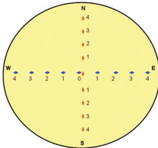
Figure 2. Diagram of the composite specimen with Knoop hardness measurements made in 1-mm increments in all four directions from the center.
