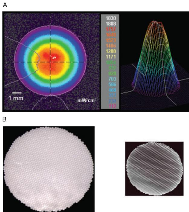
Figure 4. A, Two- and three-dimensional beam profiles across the turbo light guide tip (0 mm) (Top Hat factor = 0.610) and corresponding irradiance values ( $mW/cm^2$ ). Total irradiance (white circle) =  $716 mW/cm^2$ . B, Images of the proximal and distal ends of the turbo light guide.
