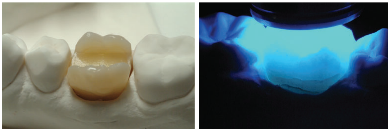
Figure 1. Experimental setup during adhesive steps. Teeth were fitted in a stone model in order to simulate neighboring teeth and their relative influence on the air flow during adhesive procedures (left). Final application and curing of the restorative material (right). Note the development of horizontal cracks at the lingual cusp base.
