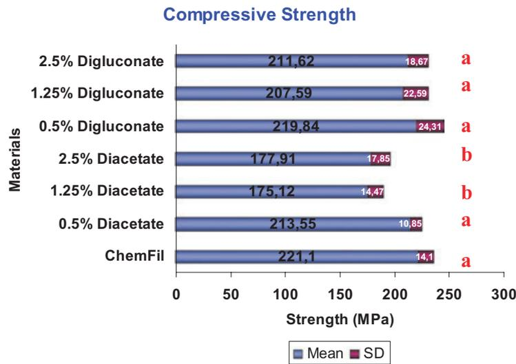
Figure 5. Mean and SD of the compressive strength of the different groups. The different letters indicate statistically different groups.
