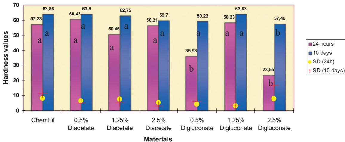
Figure 4. Mean and SD of the hardness of the different groups.
