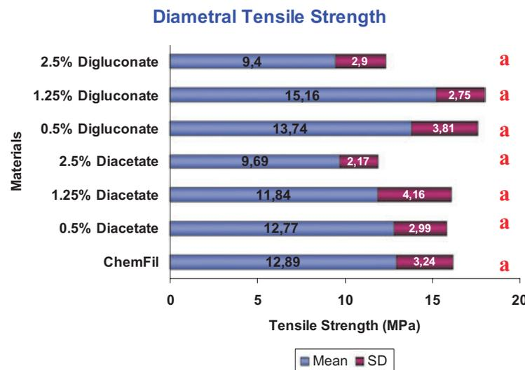
Figure 6. Mean and SD of the diametral tensile strength of the different groups. There were no differences between the groups.
