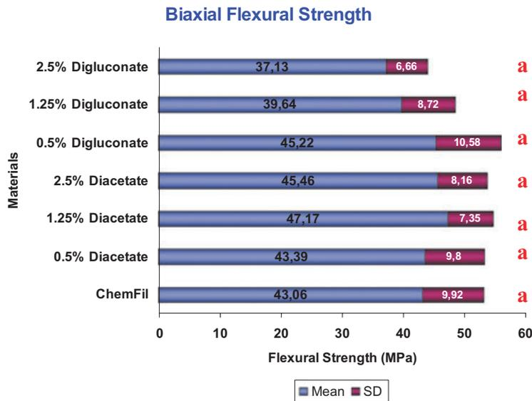
Figure 7. Mean and SD of the biaxial flexural strength of the different groups. There were no differences between the groups.
