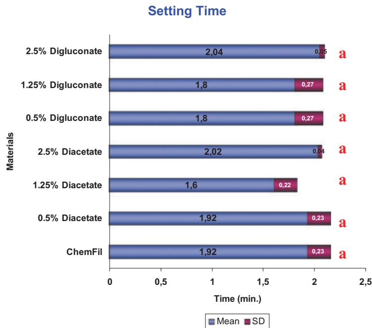
Figure 9. Mean and SD of the setting time of the different groups. There were no differences between the groups.
