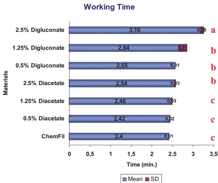
Figure 8. Mean and SD of the working time of the different groups. The different letters indicate statistically different groups.
