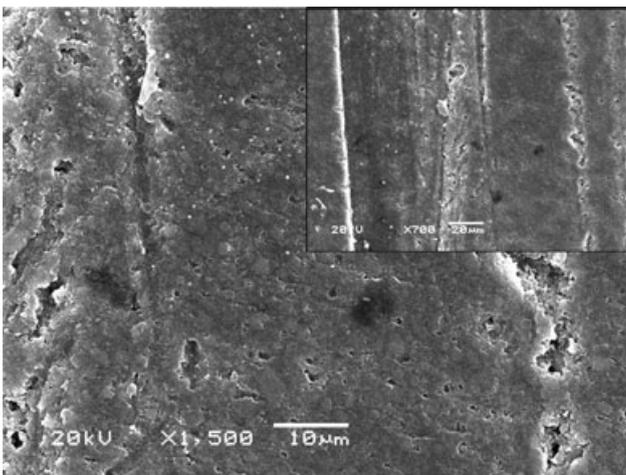
Figure 4. Scanning electron microscope image of Filtek P60 finished by Fini system.
