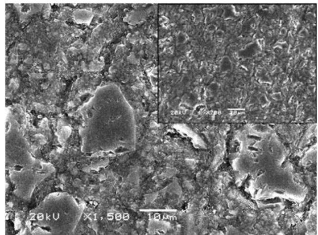
Figure 5. Scanning electron microscope image of X-tra fil finished by Flexidisc/Flexiwheel system.
