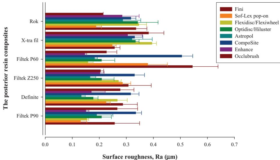
Figure 1. Surface roughness finish (Ra) of each posterior resin composite at a given finishing/polishing system.
