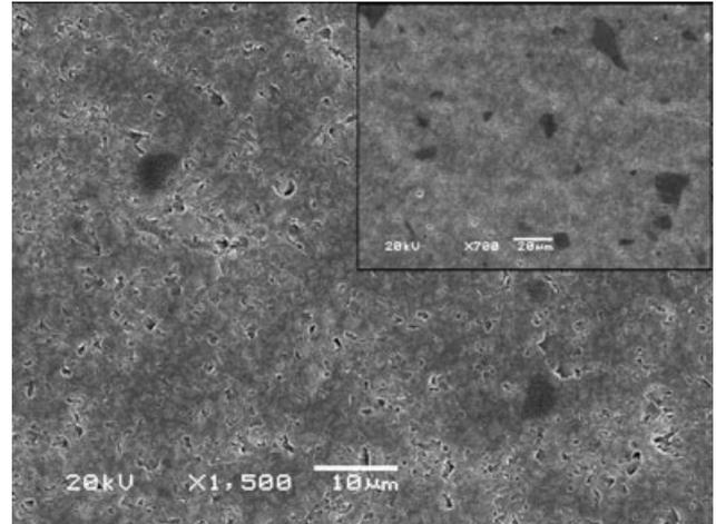
Figure 3. Scanning electron microscope image of Definite finished by Astropol system.
