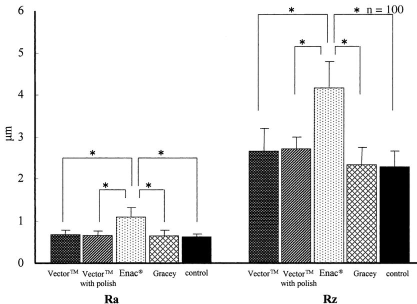
Fig. 2. Mean Ra (JIS B 0601, 1994) and Rz (JIS B 0601, 1994) values for each group. Mean Ra and Rz values for the Enac® were significantly higher than for the other groups. \**p*-value < 0.05.
